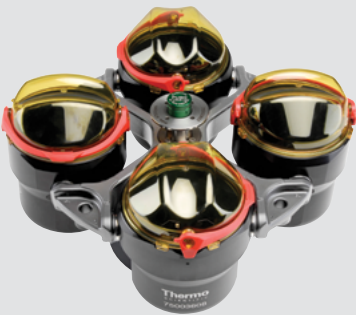
TX-750 Swinging Bucket Rotor 1 , 90°, R max 195 mm
